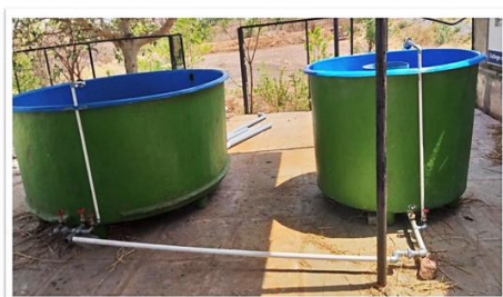
FRP Hatchery set up
