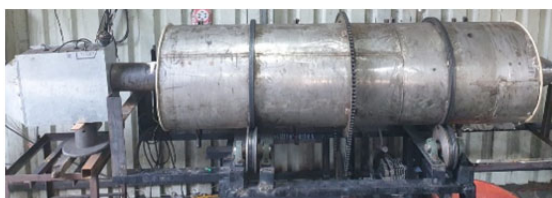
Rotary Dryer with a heater and air blower
